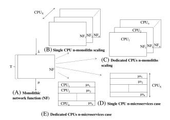
Fig. 1. Network Function (NF) Deployment
